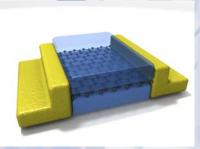
Two-dimensional materials such as graphene can achieve spectacular performance but are highly sensitive to disorder from the environment. We have developed techniques to controllably 'stack' graphene on insulating hexagonal boron nitride, which dramatically reduces disorder and increases performance. In addition, these heterostructures can display novel behavior due to the presence of 'superlattice' potentials arising from the graphene-BN stacking. In recent work, we have extended these
