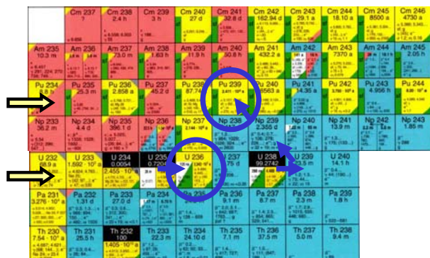
Fig. 1. Zoom into the chart of nuclides [12] relevant for neutron capture on ^{235}\text{U} and ^{238}\text{U} . Long-lived ^{236}\text{U} ( t_{1/2} = 23.4 Myr), and the decay product of ^{239}\text{U} ( t_{1/2} = 23.5 min) and ^{239}\text{Np} ( t_{1/2} = 2.36 days), the long-lived ^{239}\text{Pu} ( t_{1/2} = 24 kyr), were measured by AMS.
