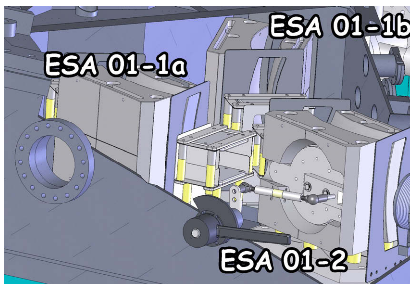
Fig. 2. 3D-view of the ESA switcher vessel. The name tags are explained in Fig. 1. The shields preventing leakage of the electric fields at the path of the ions are not shown. Ions coming from source S1 (upper left) are bent 45° by 'ESA 01-1a' and can pass through 'ESA 01-2' having its door opened. If the ions come from source S2 (upper right), they are bent 45° twice, by 'ESA 01-1b' and 'ESA 01-2' shown its door closed. The lid of the ESA switcher vessel has got a window allowing for visually checking the proper position of the door. The vessel has also got some additional ports of different dimensions so that additional devices (e.g. a beam attenuator assembly) can be brought into the ion beam's path.
