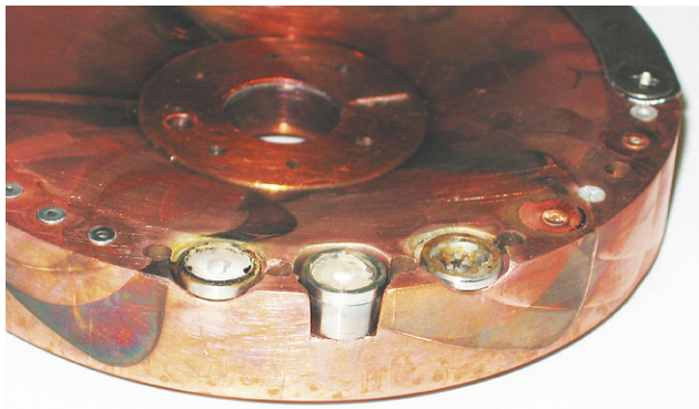
Fig. 6. Modified target holders for AMS with ^{36}\text{Cl} after usage.
